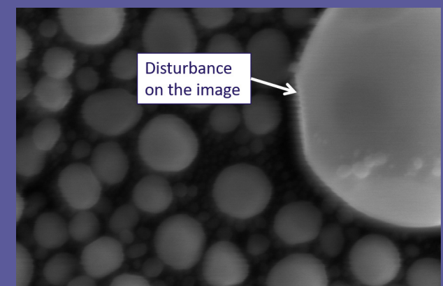
Figure 1: Vibration, magnetic fields, and acoustic noise can result in disturbance or edge noise on an electron microscope image
