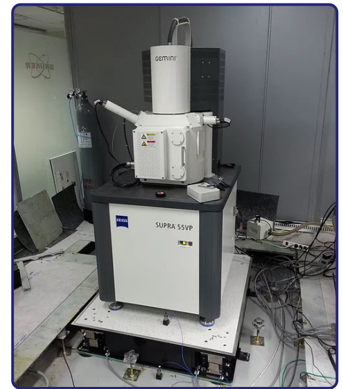
At installation, VEC tunes the DVIA-M control systems based on the data recorded during the site survey.
